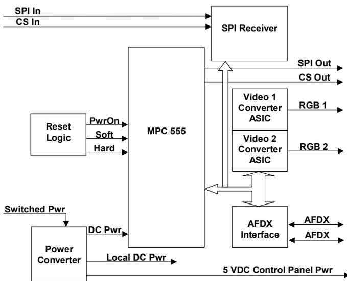
Figure 5. RMS Computer Block Diagram
