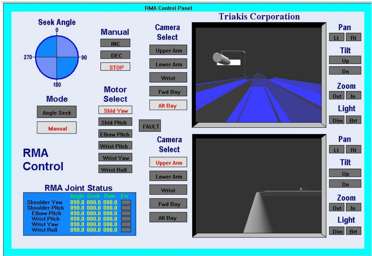
Figure 3. Simulated operator control panel ES
