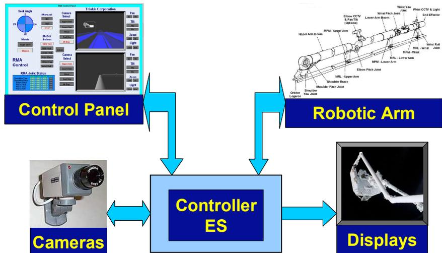
**Figure 2. ES-based simplified shuttle RMS system-level diagram**
