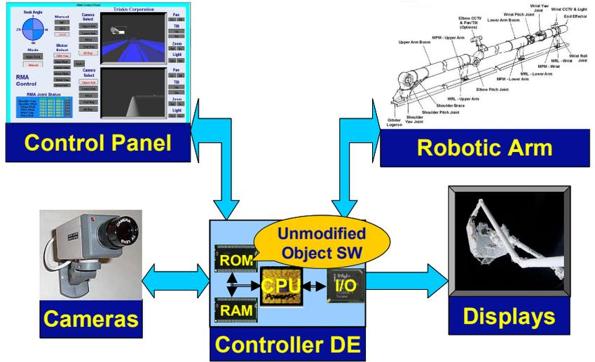
Figure 6. Testing software in system-level simulation
